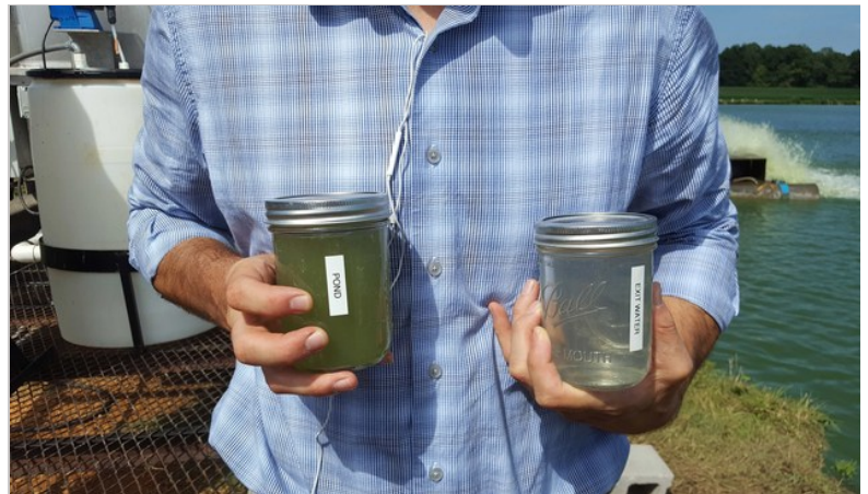
The jar on the left shows water scooped up from the pond before the water is filtered by the mobile harvesting unit. The jar on the right shows what the clean, filtered water looks like as it is pumped back into the pond.
